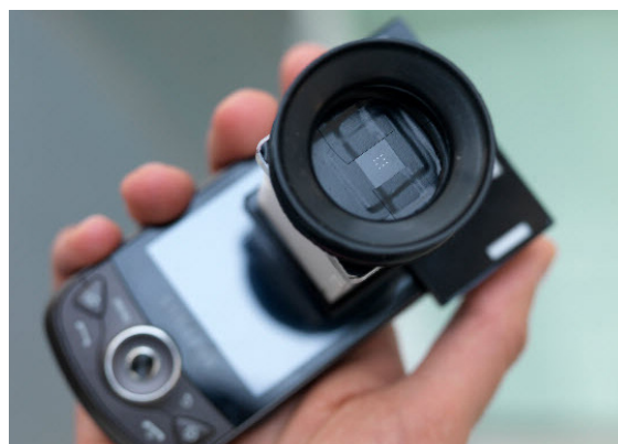
Figure 6. Netra-G: smartphone refraction, early prototype
